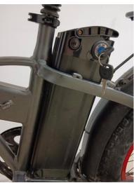
It is necessary to insert the aluminum strip of the slideway into the battery box. Figure 2 shows that the battery box is completely placed in the battery compartment
