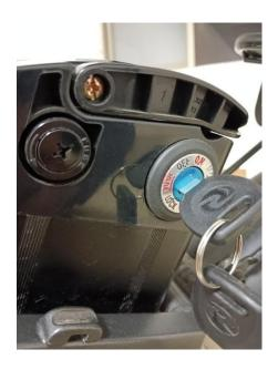
Lock position corresponding to the key: no power supply, the battery can be pulled out; (The key shall be pressed down when the lock position is switched to the off position, the same is true when the off position is switched to the lock position)
