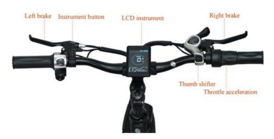
Long press(1 second) Power Button when the display is off, display, the display is fully displayed and starts to work, the power of the controller is turned on;
