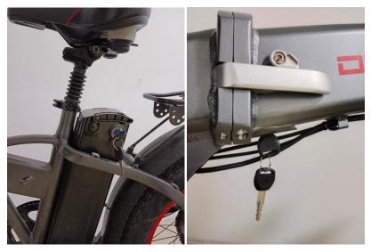
The batteries of some models need to be installed by you. Put them directly in the way shown in the picture, and then open the power lock to use.
