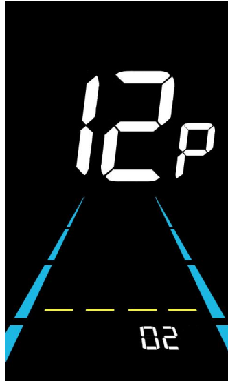
Figure 6-12 Pedal assist Start-up intensity setting interface
