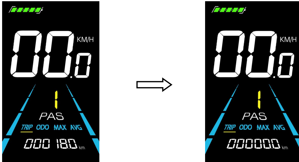
Figure 7-2 Trip Odometer Reset Interface
