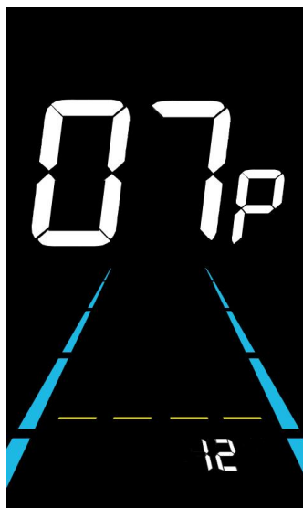
Figure 6-7 Number of speed sensor magnets setting interface
