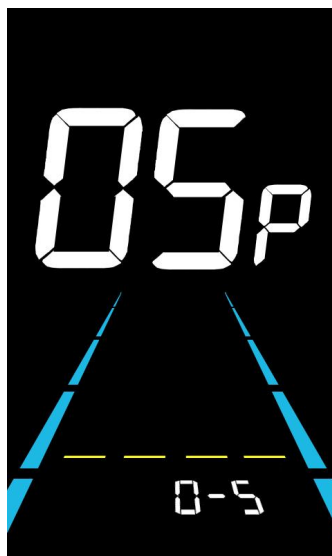
Figure 6-5 PAS level setting interface
