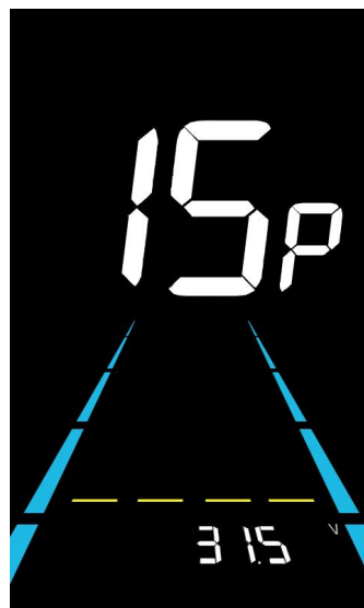
Figure 6-15 Battery under voltage value setting interface
