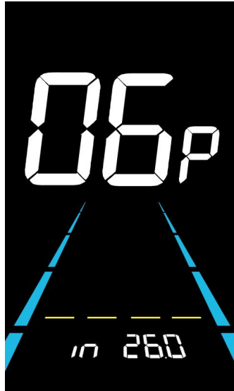
Figure 6-6 Wheel diameter setting interface
